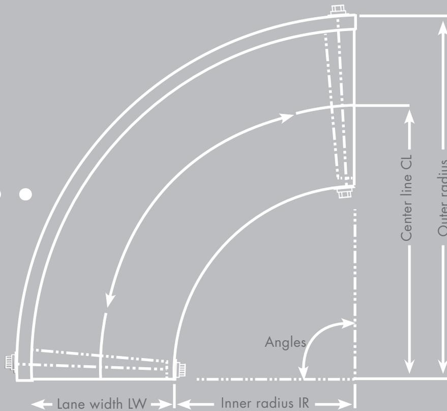
The belts run via idler pulleys, which can lead to a failure in case of a parcel jam on these curves. As a result, not only the belt, but also the expensive idler pulleys will have to be replaced.
